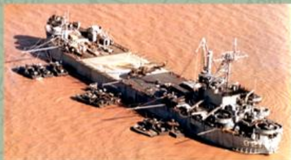
PBRs berthed alongside the tank landing ship USS Hammott County (LST 821). LSTs anchored in rivers served as floating bases for PBRs and helicopters attached to Task Force 116, providing food, berthing, maintenance, and supplies, among other services (USN photo)
