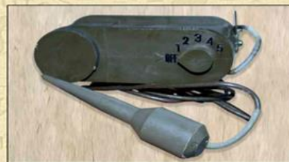
The Patrol Seismic Intrusion Detector uses a spike (seismic sensor) inserted into the ground by hand to guard a patrol's camp perimeter. The small box contains a battery, transmitter, and antenna. The transmitter indicates nearby vibrations picked up by the sensor. The vibrations are transmitted over a long wire (over 200 yards). Each spike (sensor) transmits a different beep providing the operator with a clear indication of the enemy's location and movement. (Secretary of Defense Graphics)
