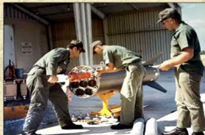
U.S. Air Force personnel load acoustic sensors into a rearward firing dispenser. July 1968 (National Archives)
