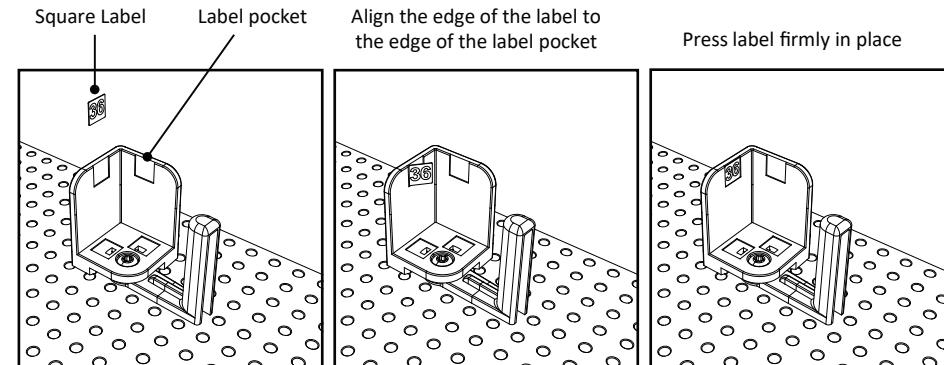
**Placing an I.D. Label onto a tool:**
