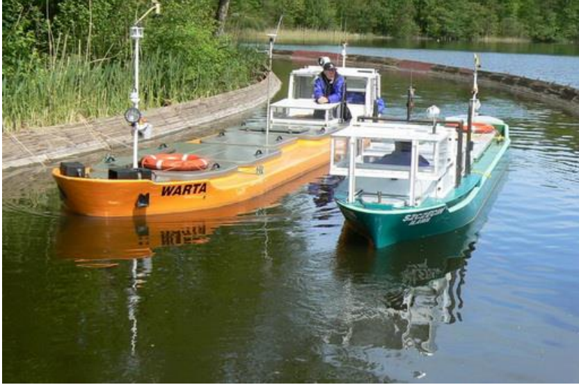
Figure 2. Training and Manned Model Simulators (MMS) for Ship Applications in a Canal ( www.ilawashiphandling.com.pl )
