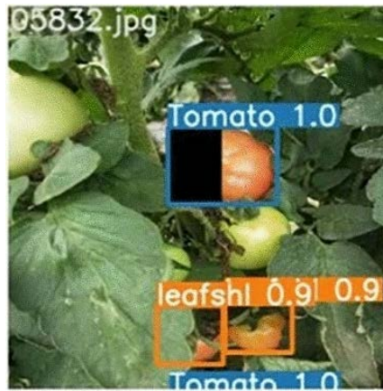
Figure 5. Tomato identification using real-time image enhancement on a harvesting robot
