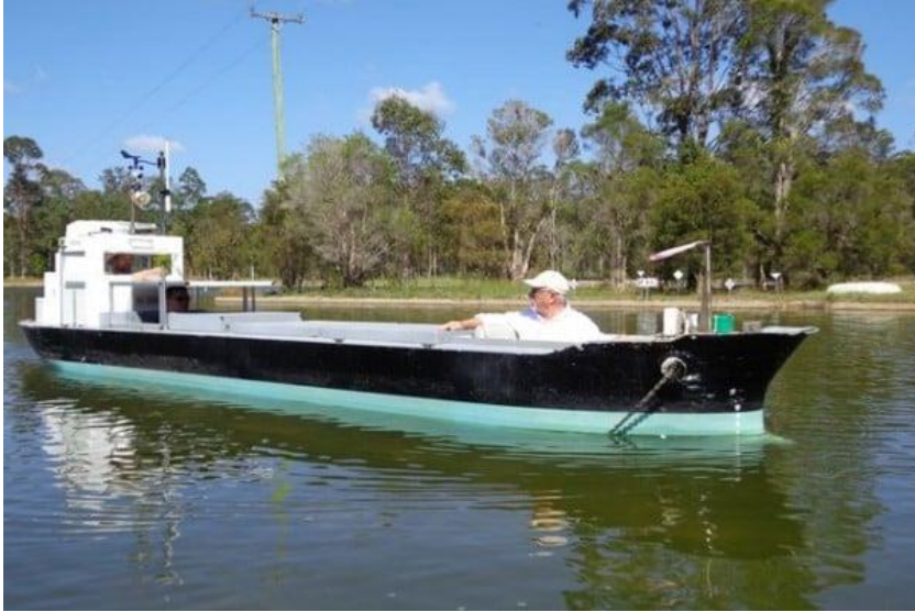
Figure 3. Training and Manned Model Simulators (MMS) for Bulk Carrier Ship Applications ( https://www.portrevel.com/ )
