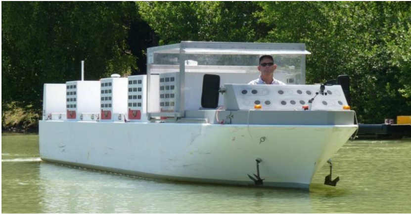
Figure 1 Training and Manned Model Simulators (MMS) for Ship Applications ( https://www.portrevel.com/ )
