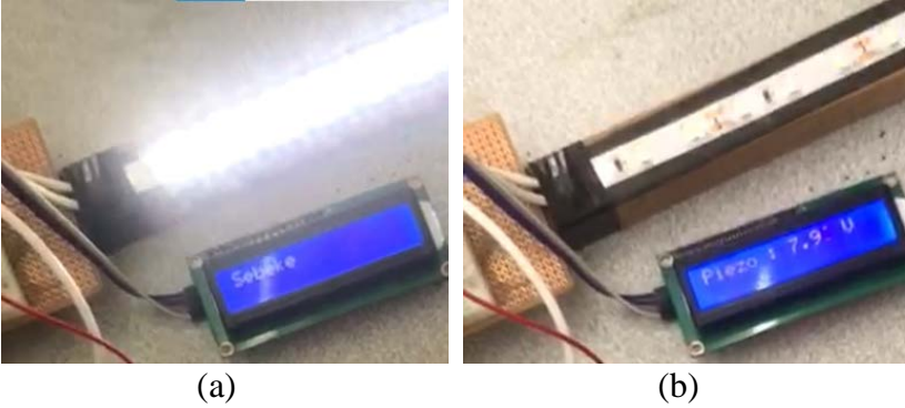
Figure 12. (a) Lighting Mains Supply, (b) Supply With Piezoelectric Energy Harvesting
