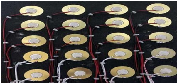
Figure 11. Positioning of Transducers in the System
