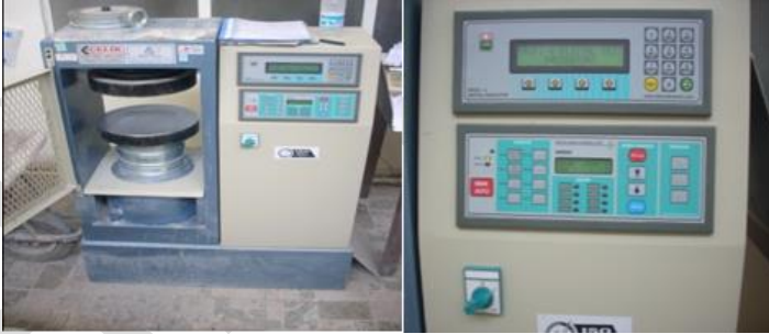
Figure 3. Device for pressure testing
