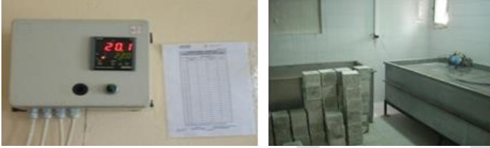
Figure 4. Curing concrete samples
