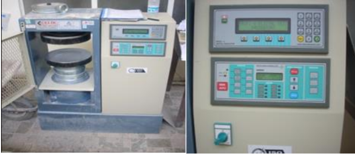
Figure 3. Device for pressure testing
