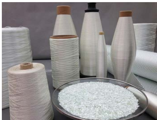
Fig. 5. Boron glass wool and textile type glass fiber [14]
