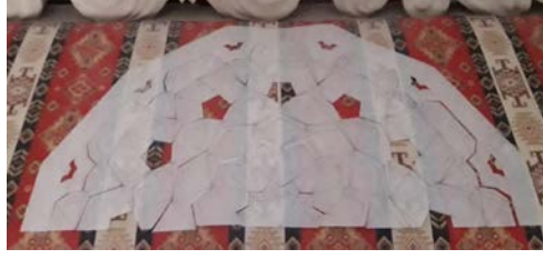
Figure 3. Muqarnas molds made of polyester press tape
