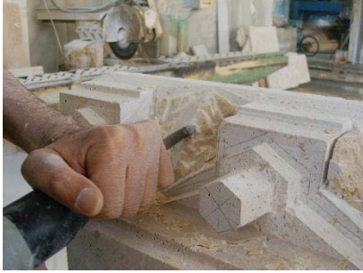
e) Detailing muqarnas units with compressed air hammer
