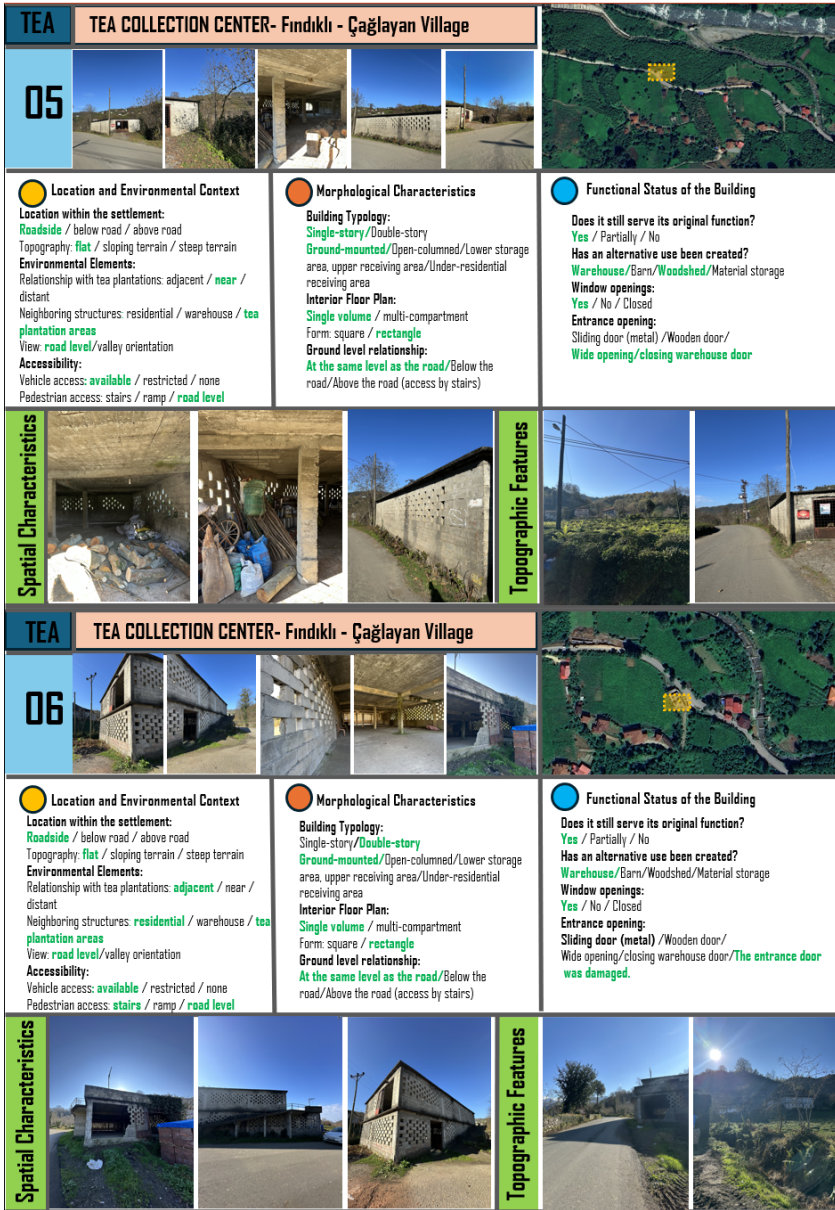
Figure 10. Spatial analysis data sheets of tea collection points (05–06) (Elaborated by the authors)
