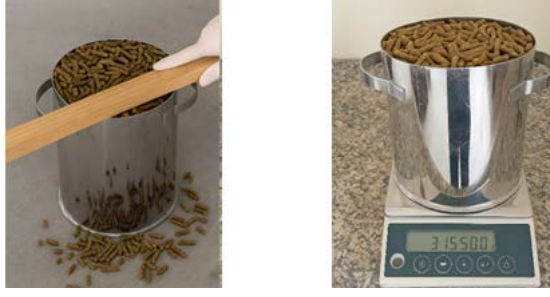
Figure 2. Procedure for Determining Pellet Bulk Density
