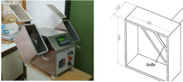
Figure 4. Mechanical durability testing apparatus and cage dimensions
