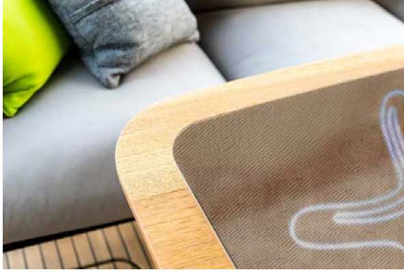
Figure 5. Flax fiber coated with epoxy detail in the deck table of The Sunreef Yachts Eco Project (Sunreef Yachts, 2023).
