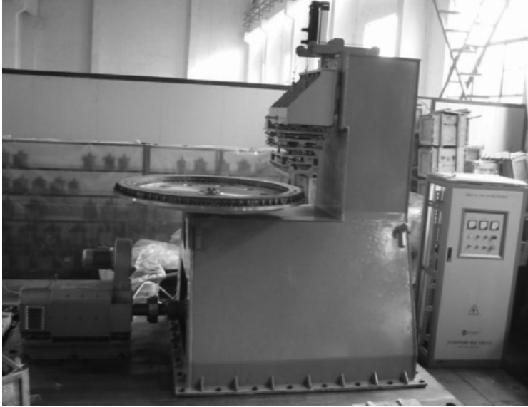
Figure 8. The Photo of the Superconducting Dynamic Magnetic Levitation Force Measurement System (SCML-03) [16_].
