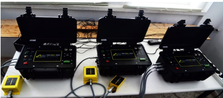
Figure 3. Dynamic Data Collection Device and Acceleration Recording System
