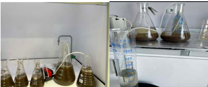
Figure 1. Batch activated sludge system
