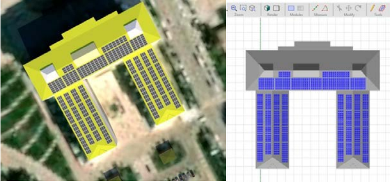
Figure 2. a) Modeling the facility in Sketchup program, b) Modeling the facility in PVsyst program
