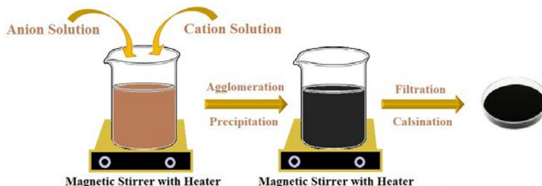
Figure 4. Co-Precipitation Method in Production of Metal Oxide Nanoparticle
