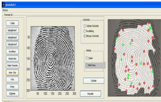
Figure 8. Fingerprint that has been cleaned and freed from faulty feature points
