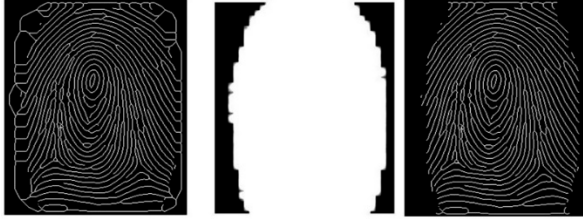
Figure 5. Cleaning the thinned image using thinning process and area image mask
