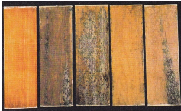
Figure 5. Wood samples with and without UV stabilizer (Evans et al., 2015).
