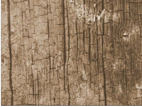
Figure 8. Surface degradation of wood (Babar & Kathryn, 2020).
