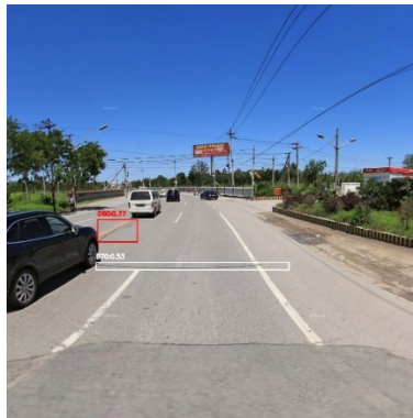
Figure 17. The result of the customized YOLOv8n model with transfer learning, TTA, and NMS applied on a sample test image from the RDD2022 dataset
