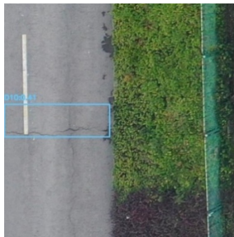
Figure 23. The result of the customized YOLOv8l model with transfer learning, TTA and NMS applied on a sample test image from the SVRDD dataset.
