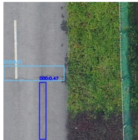
Figure 19. The result of the customized YOLOv8n model with transfer learning, TTA, and NMS applied on a sample test image from the SVRDD dataset.
