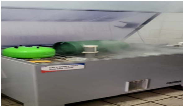
Figure 14. Salt Spray test setup (Alper,20005)
