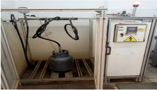
Figure 13. Compressive fatigue test setup (Alper,2025)
