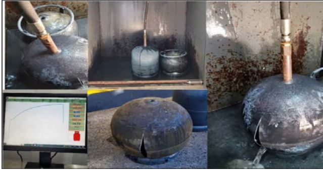
Figure 12. Bursting pressure test setup(Alper,2025)
