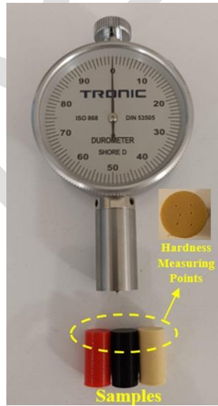
Figure 2. Hardness measurement with durometer
