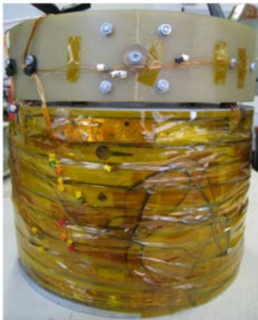
Figure 4. Prototype SFCL coil prior to installation in cryostat [17]
