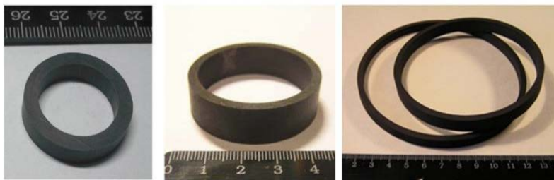
Figure 7. Some tested \text{MgB}_2 rings of various sizes [27]
