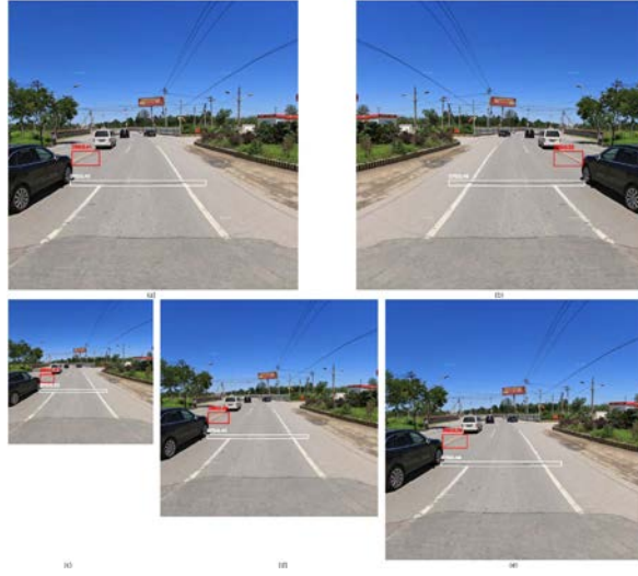
Figure 16. The results of the customized YOLOv8n model with transfer learning and TTA applied on a sample test image from RDD2022 dataset (a) The result obtained with the original image (b) The result obtained with the image symmetrically mirrored from left to right (c) The result obtained with the image set to 50% of the original resolution (d) The result obtained with the image set to 75% of the original resolution (e) The result obtained with the image set to 90% of the original resolution
