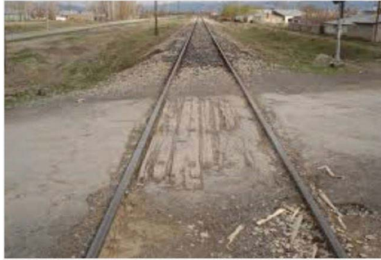
Figure 3.1. Example of an at-grade crossing without barriers and without a guard (completely uncontrolled) (Bozlioğlu 2017)
