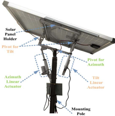
Figure 5. solar tracking angles and mechanical structure of the dual-axis solar tracking system (Hammam et al., 2025)
