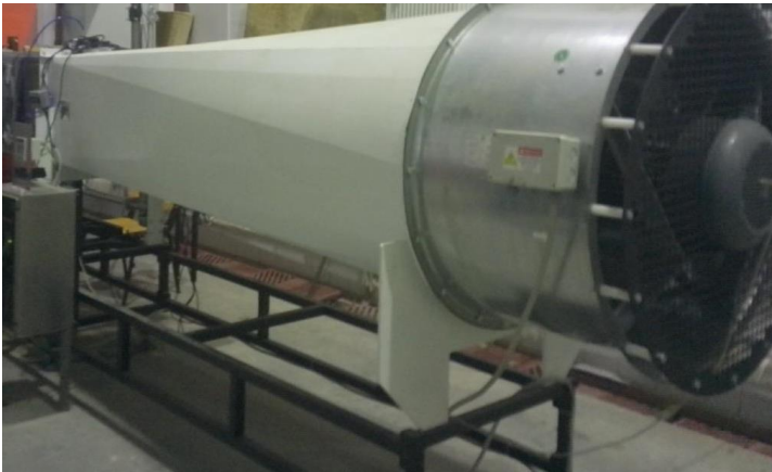
Figure 5. Wind tunnel diffuser and fan section
