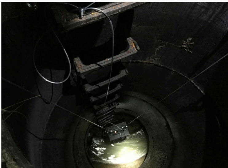
To more easily sample sewage from multiple locations before it reaches a treatment plant, MIT scientists designed sophisticated robots that can be lowered into manholes dotted throughout a community. Image credit: Biobot Analytics.
