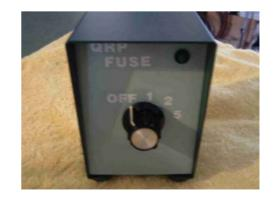
fuses and the reset for the 5-amp circuit breaker. I also included an LED on the output side of the unit to Delta Amateur Radio Club
