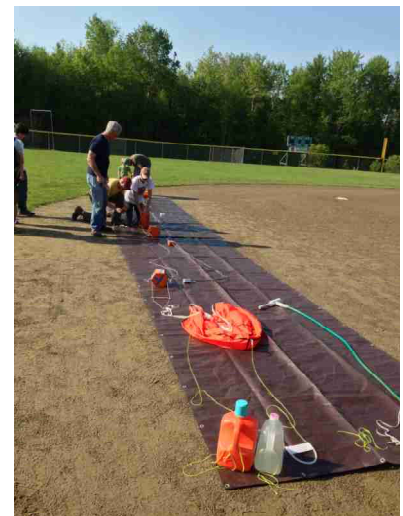
(1) Richard Eason AA1PJ oversees preparation for the balloon launch. The balloon is attached to the U-hook in near field. Then the parachute with repeater after it. Note the J-pole antenna attached to the string. Then the temperature, CO 2 and UV sensor package.
