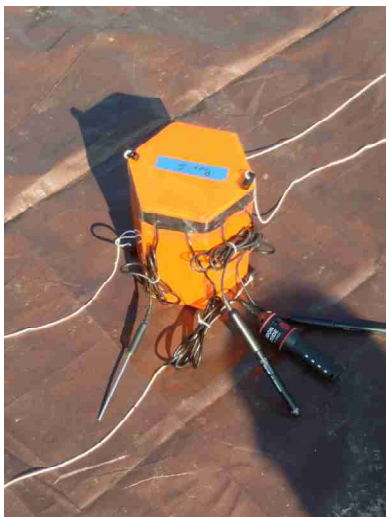
(2) The temperature, CO 2 , and UV sensor package
