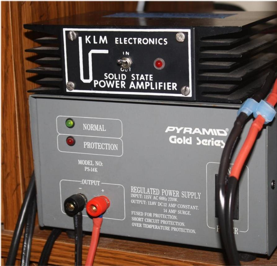
In this photo, the ring terminals on the new cable go to the power supply and the amp's power leads connect to the other end of the new cable.
