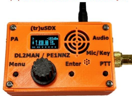
(tr)uSDX 5-band Multimode QRP
