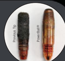
Tip comparison after one full shift of heavy welding*
