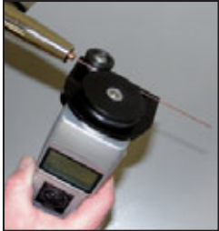
HHSS-12 WIRE FEED SENSOR for readings at torch
