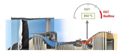
c. EGT Margin (EGTM) is the difference between the peak EGT incurred during take-off and the certified redline EGT. It is used to evaluate and track engine time on-wing & health.
