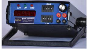
By using a four-wire, Kelvin-based, resistance measurement system, the Model 5012-06XP eliminates the inaccuracies intro-
