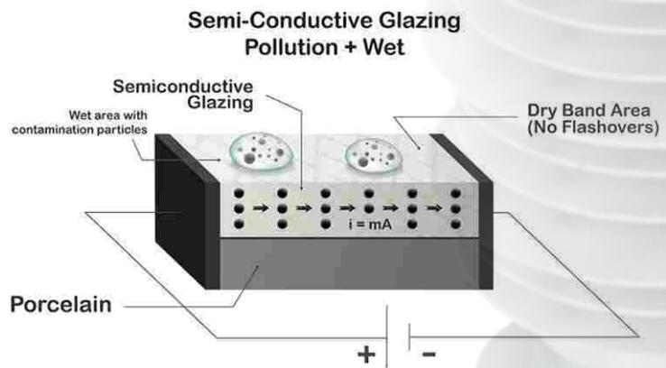
Figure 4. Semi-conductive Glazing Principle of operation
