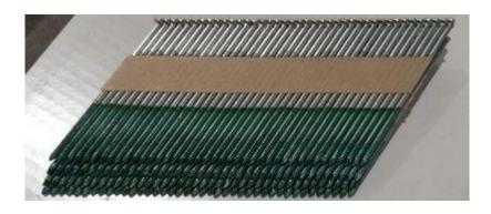
**D-head paper tape** framing nails are joined by a strip of paper and glued using the same technique as joist hanger nails. Our paper tape is 100% waterproof and designed for outdoor use, which means that nails will remain in their position in any weather conditions. Due to its D-shaped head, it is possible to glue nails without gaps which means more nails per strip. This type of nail ensures convenient work with a nail gun in tight situations.
