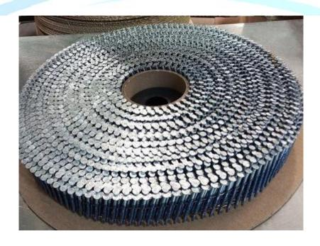
**Jumbo coils** are manufactured in a flat coil with a plastic axle and paper cover. On smaller Jumbo coils the cover and axle are not used. Jumbo coil nails are used in automatic pallet forging machines. In such coils the number of nails may range from 450 to 3000 nails per coil. These nails are designed to be used with a pneumatic nail gun and come in long, coiled strips that can hold up to 3000 nails.
