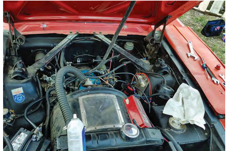
ABOVE: The RC2-60 engine before removal for a rebuild. Notice the large fan shroud.
