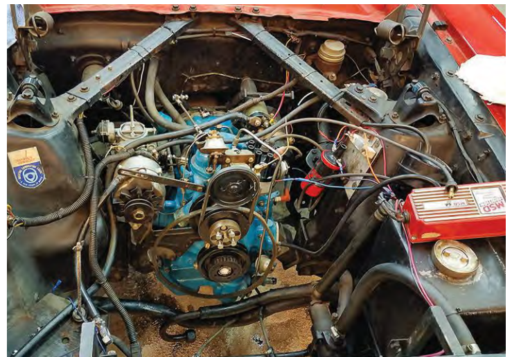
BELOW: With the fan shroud removed, you can get a better view of the RC2-60 Wankel engine. The engine had been refurbished at least once before and some components, like the newer MSD ignition box and coil, were not part of the original test configuration.
