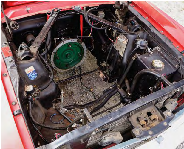
ABOVE: The engine compartment reveals several modifications for the RC2-60 engine, including fabricated motor mounts, transmission bellhousing adaptor, and brackets for a larger radiator.
