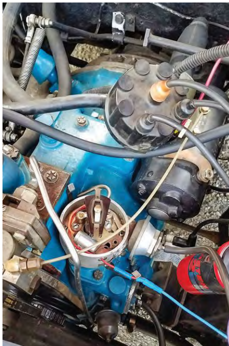
For the dual-rotor engine’s pair of spark plugs, only two of the V8 distributor ports are used.
