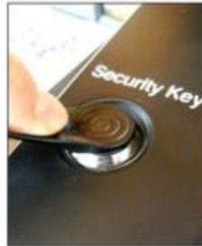
**2** Press the Security Key onto the pad and hold firmly.
