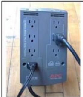
**1** With Lid removed plug the tabulator power cord into an outlet.
