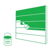
4 Caulk at all end joints and the corners of wall. Clean up the plank before painting.
