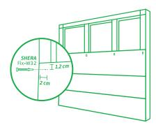
3 Fasten the plank to steel studs, with one on top of the other, from bottom of the wall to the top.
