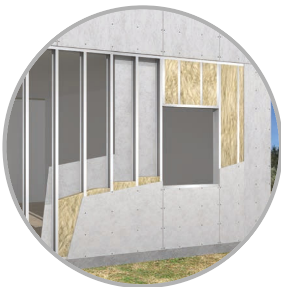
100mm wall 100mm insulation U-VALUE = 0.322 w/m 2 k
