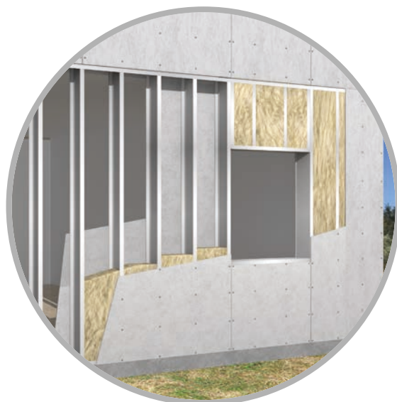
200mm wall 200mm insulation U-VALUE = 0.168 w/m 2 k
