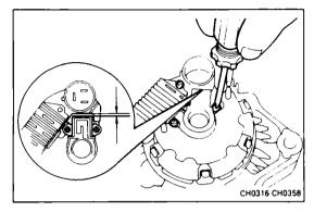
(c) Install the five screws until there is a clearance of approx. 1 mm (0.04 in.) between the brush holder and connector.
