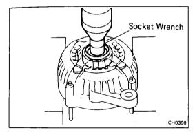
(b) Using socket wrench and press, press out the bearing.
