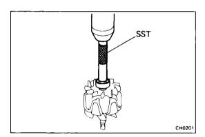
(b) Using SST and a press, press in a new bearing and bearing cover.
