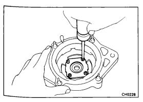
(d) Install the bearing retainer with the four screws.
