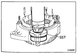
(c) Using SST and a press, press in a new bearing. SST 09608-20012 (09608-00030)
