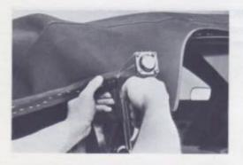
(b) Tack top cover to belt tacking strip starting from top cover inner verticle edge reference mark on tacking strip assembly towards the front.
