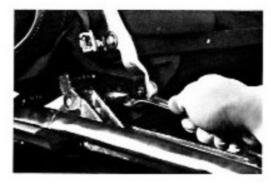
(c) Remove the bolts on each side retaining the No. 1 bow front side rail to the center side rail and remove the No. 1 bow.
