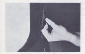
(c) Detach the headliner from the No. 4 bow. Pull to break cement bond.
