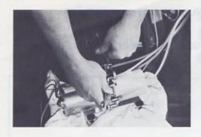
(e) Disconnect the hydraulic lines from the motor and pump assembly and cap the open fitting to prevent leakage of fluid.
