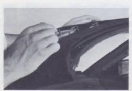
INSTALL WINDSHIELD HEADER EXTENSION MOLDING Install the extension molding and the six nuts.
