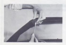
(c) Remove the plastic retainer at the upper end securing the weatherstrip to the "A" pillar.
