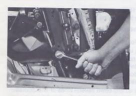
3. REMOVE TOP STACK HYDRAULIC CYLINDER
