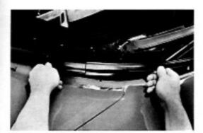
(d) Raise the moldings off body and disengage the quarter belt moldings from the back belt moldings.
