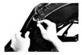
(f) Align sides of top cover with side rails and secure top cover flaps to the front rails.
