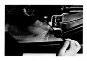
(b) Connect the regulator arm to the glass bracket assembly with the pin and spacer.
