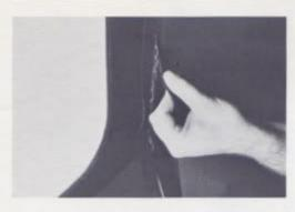
(c) Attach headliner to No. 4 bow. Starting at center working toward each end, pull headliner rearward while attaching to pull out wrinkles.
