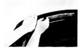
(g) Raise the top and latch it to windshield header. Check appearance of top cover, top operation and latching effort of top.
