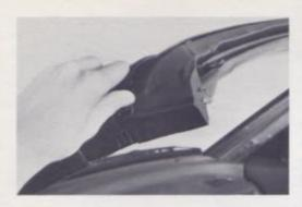
INSTALL WINDSHIELD HEADER MOLDING CAP Install the molding cap and the nut.
