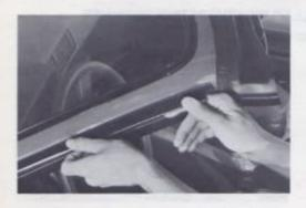
REMOVE "A" PILLAR DRIP MOLDING Pull off the "A" pillar drip molding.
