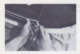
(b) Mark the location of the inner vertical edge of the top cover backlite opening on the belt tacking strip assembly.
