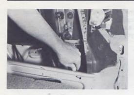
3. HOOK HEADLINER STRAP TO AUXILIARY "B" PILLAR BRACE
