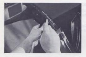
(b) Mark the location of the belt tacking strip, upper and lower edge, on the outer surface of the rear stay pads. Mark the location of the inner vertical edge of the stay pads on the outer surface of the backlite.
