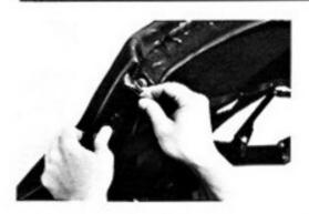
(c) Align sides of top cover with side rails and install top cover flaps to the front rails.
