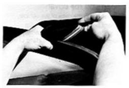
(d) Detach top material from the No. 4 bow by pulling the No. 4 bow feature strip out of the No. 4 bow feature strip retainer.
