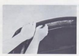
(g) Raise the top and latch it to windshield header. Check appearance of top cover, top operation and latching effort of top.
