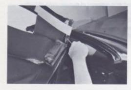
(b) Lower the top halfway and install the end of the cable into the front side rail with the screw.
