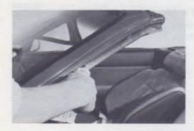
(e) Apply a continuous bead of black weatherstrip adhesive to the channel of the "A" pillar weatherstrip retainer.
