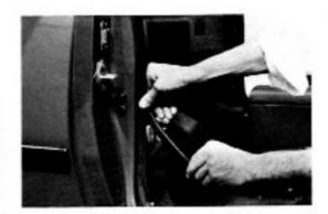
3. REMOVE LOCK PILLAR WINDLACE FROM LOCK PILLAR PINCH WELD FLANGE
