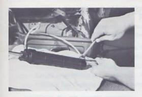
(d) Disconnect the hydraulic lines from the cylinder and remove the cylinder.
