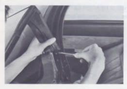
(d) Continue removing the weatherstrip from the front header retainer, using a suitable release agent, gently pull the weatherstrip out of the retainer while inserting the flatbladed tool between the weatherstrip and the weatherstrip retainer to break the cement bond and remove the front header weatherstrip assembly.
