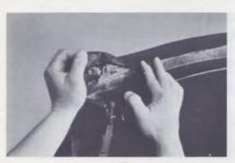
DETACH TOP COVER FROM NO 1. BOW Pull top cover to break cement bond.
