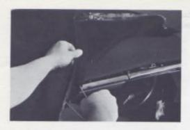
REMOVE SIDE RETENTION CABLE FROM TOP COVER
