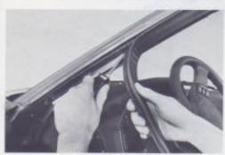
(b) Using a suitable release agent (Kent special releasing agent or equivalent) and a flat-bladed tool, grasp the lower end and gently pull the weatherstrip out of the retainer while inserting the flat-bladed tool between the weatherstrip and the weatherstrip retainer to break the cement bond.
