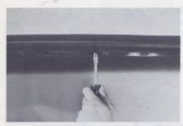
REMOVE WINDSHIELD HEADER EXTENSION MOLDING
