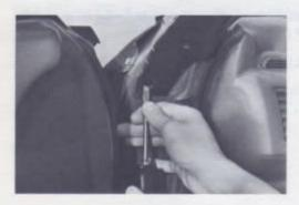
(h) Install the two plastic retainer clips to the lower end of the weatherstrip.
