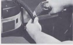
(d) Check tension of the stay pad between the No. 1 and 2 bows. No. 2 and 3 bows and No. 3 and 4 bows.
