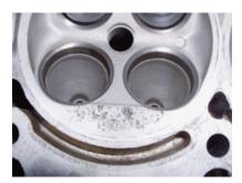
Using poor quality fuel also allows detonation & this is more common if boost is increased (by any amount) & or the cylinder head has been shaved. The factory knock sensors are not
