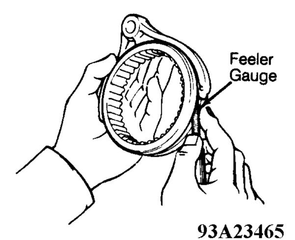
**Fig. 11: Measuring Shift Fork & Synchro Ring Assemblies (2 Of 2)** Courtesy of TOYOTA MOTOR SALES, U.S.A., INC.
