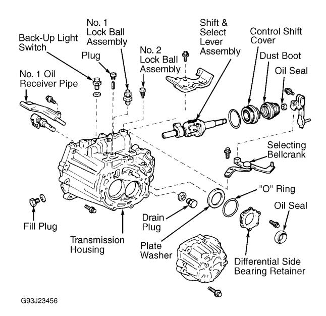
**Fig. 4: Exploded View Of Transmission Assembly (2 Of 3)** Courtesy of TOYOTA MOTOR SALES, U.S.A., INC.
