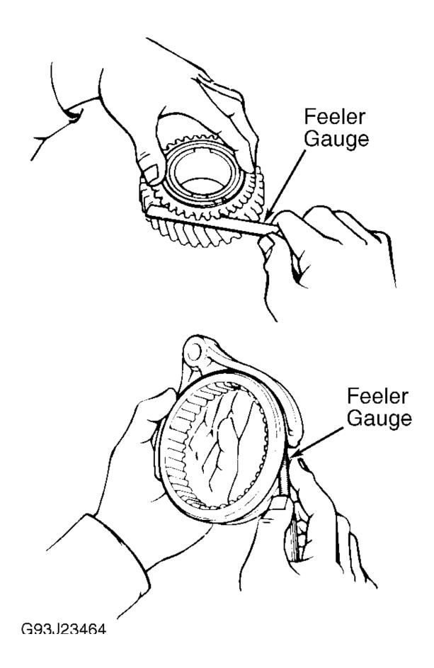
**Fig. 10: Measuring Shift Fork & Synchro Ring Assemblies (1 Of 2)** Courtesy of TOYOTA MOTOR SALES, U.S.A., INC.
