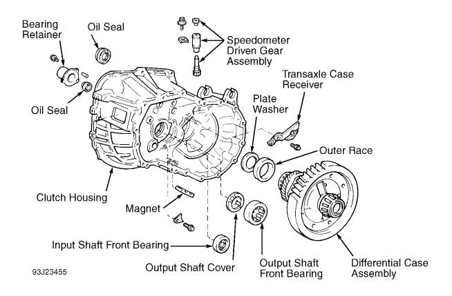
**Fig. 3: Exploded View Of Transmission Assembly (1 Of 3)** Courtesy of TOYOTA MOTOR SALES, U.S.A., INC.
