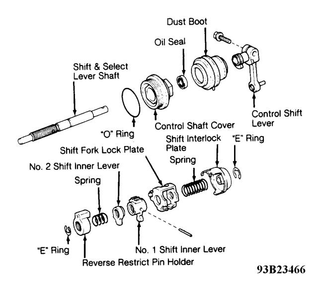
Fig. 12: Exploded View Of Shift & Select Lever Assembly Courtesy of TOYOTA MOTOR SALES, U.S.A., INC.
