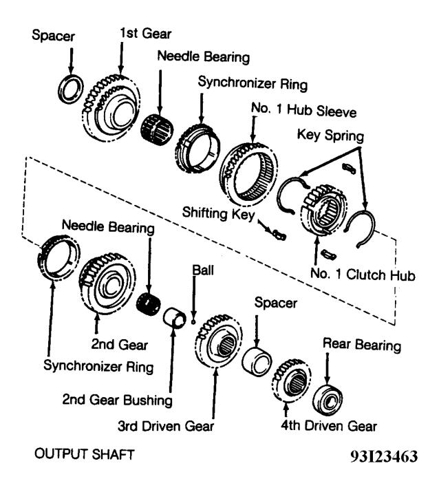
**Fig. 9: Identifying Input & Output Shaft Components (1 Of 4)** Courtesy of TOYOTA MOTOR SALES, U.S.A., INC.
