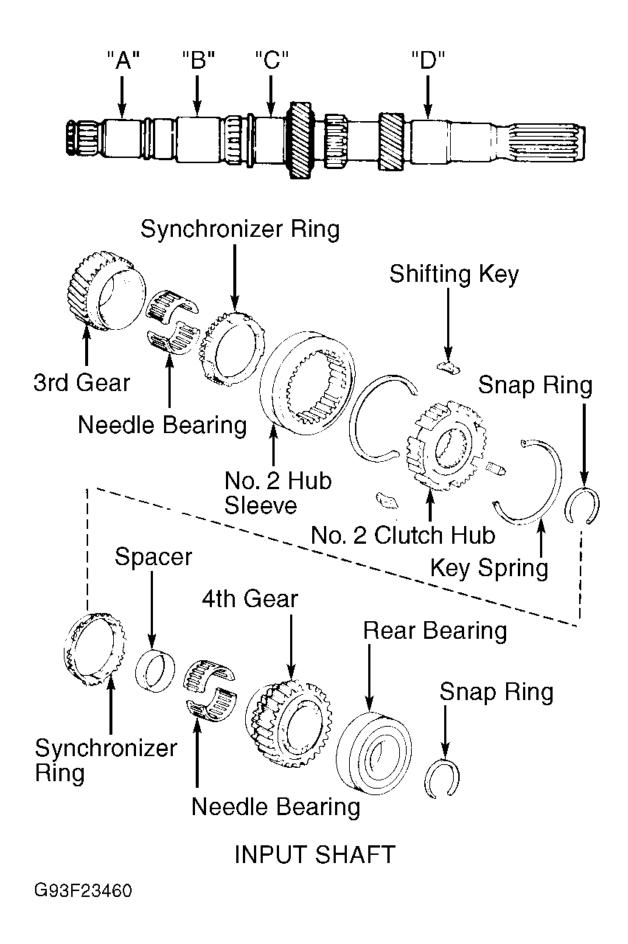
**Fig. 6: Identifying Input & Output Shaft Components (1 Of 4)** Courtesy of TOYOTA MOTOR SALES, U.S.A., INC.
