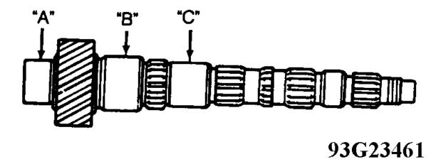
**Fig. 7: Identifying Input & Output Shaft Components (1 Of 4)** Courtesy of TOYOTA MOTOR SALES, U.S.A., INC.
