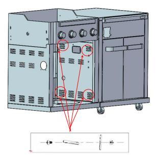
Insert the fastening clips from the bottom upwards, applying some force. This may require a bit of effort, but it ensures the units are securely connected as intended.
