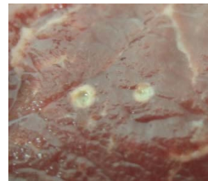
"hard" vs. "soft" with small ball using COAG current
