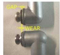
The upper prophy angle in the photo is far beyond the acceptable limits of wear. The gap, which should not exist, caused a blackened mixture of prophy paste and saliva to exude onto the patient. Compare the edge of the hub to one in the prophy angle in the lower part of the photo.
