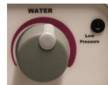
The red **Low Pressure** light next to the water knob comes on when the water flow/pressure drops below the safety point. **IMPORTANT!** Do not operate the Scaler until you have corrected the condition, and adequate supply water is again available. See pages 5 and 6 for further information. Lavage is active only in the Scaler mode.
