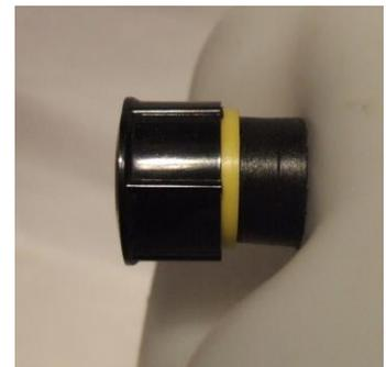
At the end of each day's use, release pressure from the tank by pulling out the button on the side of the DE-4 tank. Uncouple the quick disconnect. Note that the button may be rotated ¼ turn counterclockwise and will stay open until turned back clockwise.
